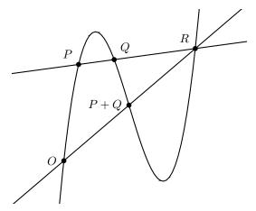
*Proof.* Define addition on E(k) by: for  $P, Q \in E(k)$ , take the intersection R of  $\overrightarrow{PQ}$  (if P = Q, take the tangent line at P) and  $E_f$ , and let P + Q be the third intersection of  $\overrightarrow{OR}$  (if R = O, take the tangent line at O) and  $E_f$ .
